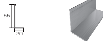
"L" 55x20 PROFILE L=3000mm FOR 300 mm STAVES
